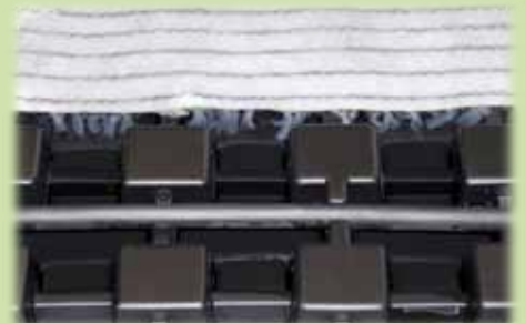
Once installed, the wicks in the wicking mat reach down into the storage cells and transport the water towards the substrate.
